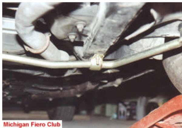
Double check everything to make sure there are not clearance problems with cables, hoses, exhaust, wiring, etc...
