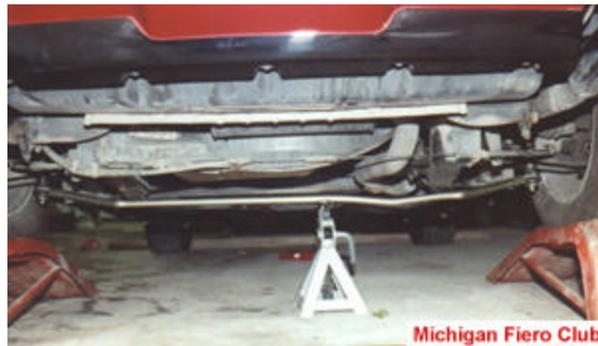
Trial fit the front frame bushing. Mark the holes in the frame and then drill out the holes with the 3/8" drill bit. Shown here is the driver's side
