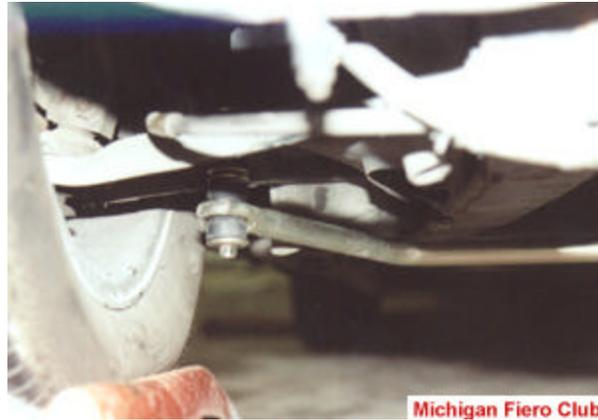
Support the sway bar, so as you can align the frame bushings.
