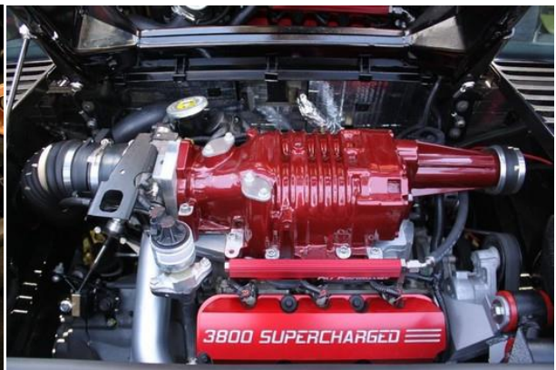
3.8 supercharged V6 in the Fiero
