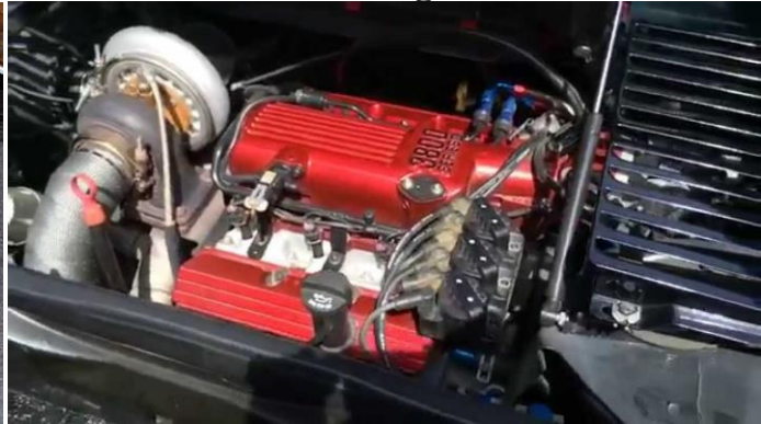
3.8 turbocharged V6 in the Fiero
