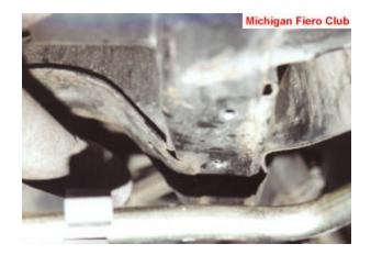
Support the sway bar, so as you can align the frame bushings.
